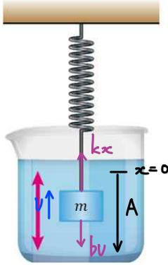
$$\begin{aligned} \Sigma F = ma &: -kx - bv = ma \\ &\quad \quad \quad \frac{d}{dt} \quad \quad \frac{d^2}{dt^2} \\ \rightarrow m \frac{d^2x}{dt^2} + b \frac{dx}{dt} + kx &= 0 \quad (\leftarrow \frac{d}{dt} = D) \\ \therefore (mD^2 + bD + k)x &= 0 \\ b^2 - 4km &\begin{cases} > 0 : \text{과감쇠} \\ = 0 : \text{임계감쇠} \\ < 0 : \text{미감쇠(진동)} \end{cases} \end{aligned}$$
